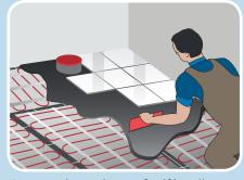
Cover with one layer of self levelling compound if needed, and allow to dry before tiling.
