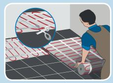
Start laying the mat. When you reach the end of the mat run simply cut the mesh and turn the mat. The red cable must NOT be cut.
