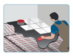
Apply flexible self-levelling compound and/or tile glue, depending on the flooring.
