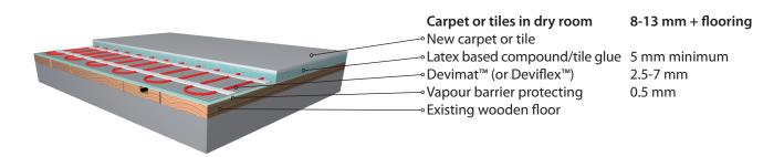
Other combinations of top flooring and existing floor construction are also optional.
