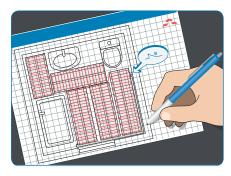
Draw a plan in order to position cable, cold tail, floor sensor, thermostat and connection box, if any. Avoid all present and future objects fixed to the floor such as toilets, bath tubs etc.
