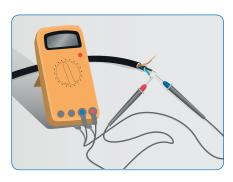
6) Check the insulation resistance and Ohm rating of the heating cables/ mats before, during and after installation. Compare the Ohm rating with the nominal, written on the cable/mat label.
