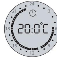
⚠ The display shows required temperature. In periods with lowering of temperature, however, the temperature will be lowered according to the set-back level (e.g. 5°C) that has been defined in connection with installation of the thermostat.
