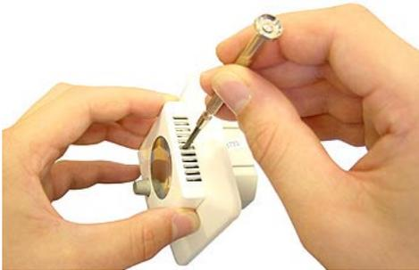
Remove the front cover by gently pressing the release tab in the top (center hole), and lift out the cover.
