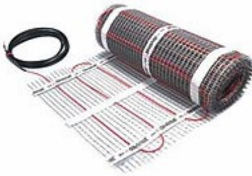
(rated 100W/m<sup>2</sup>) and one for concrete based floors (rated 150W/m<sup>2</sup>). The Devimat is made according to the highest European Standards, part of which state that the amount of heat that can be installed on to a timber floor should be limited from a point of view of safety, hence the two mat types. The self-adhesive, open weave mesh design of the Devimat, plus only having one connection tail, at the start of the mat,
