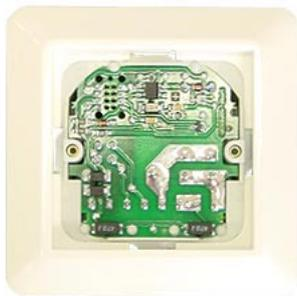
Remove the frame from the thermostat.
