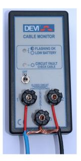
The deviguard is connected to the heating cable/mat to test the element before installation and can also be left monitoring the element until the floor/room is complete.
