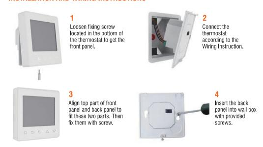
**NOTE:** Thermostat should be mounted in a standard 86 type switch box.
