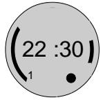
**Step 15** Save program To save programs, press and hold the button to return to the normal display. By pressing the button once you can now toggle between manual and timer modes.
