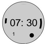
**Step 14** Continue Rotate button to indicate next warm floor start time, press the button, rotate to the end of the period and press button again. Continue this through the whole week.
