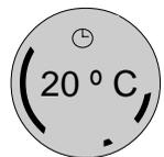
**Step 16** Set floor level The button now controls the air temperature of your **deviheat** system. The controller can be adjusted to the required air temperature on a range of 5-35°C. The displayed air temperature is what the controller will provide at the times programmed.
