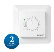
The DEVIreg™ 530 is a simple electronic thermostat with a 2-pole switch, using a floor sensor (wire) to measure and control the desired floor temperature. It can be either flush-mounted or surface-mounted.
