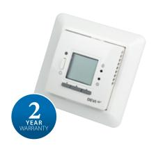
The DEVIreg™ 535 is an intelligent electronic timer thermostat with a 2-pole switch that contains three functions: floor sensor, room sensor or a combination of the two. The thermostat uses the room sensor to control the room temperature and the floor sensor (wire) to limit the maximum floor temperature.
