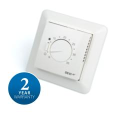
The DEVIreg $^{\rm m}$  532 is a simple electronic thermostat with a 2-pole switch , using the room sensor to control the room temperature and the floor sensor (wire) to limit the maximum floor temperature. It can be either flush-mounted or surface-mounted.
