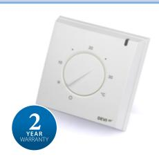
The DEVIreg™ 132 is a simple electronic thermostat to be installed directly on the wall, using a room sensor to control the room temperature and a floor sensor (wire) to limit the maximum floor temperature.
